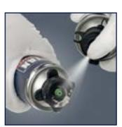
Cleaning a gun applicator of uncured polyurethane foam
